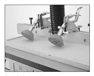
Figure 21. Pressure rollers.
